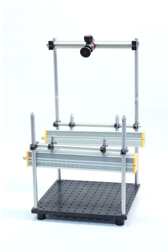
Figure 12: Camera holder post placed.
