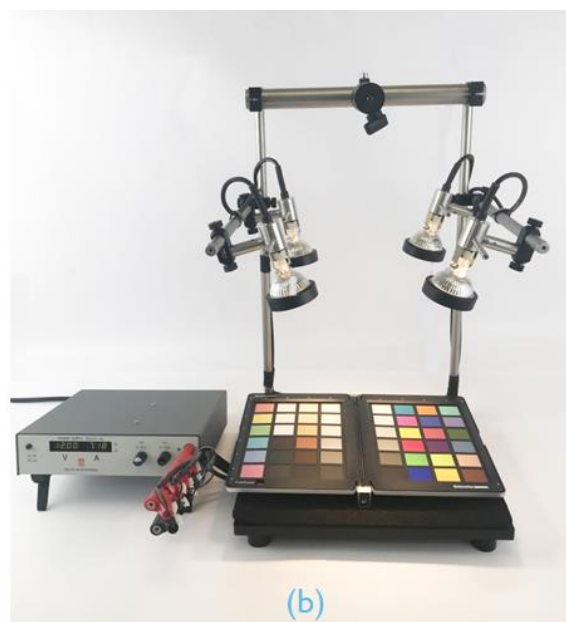
Figure 20. Test the power connection for the lamps
